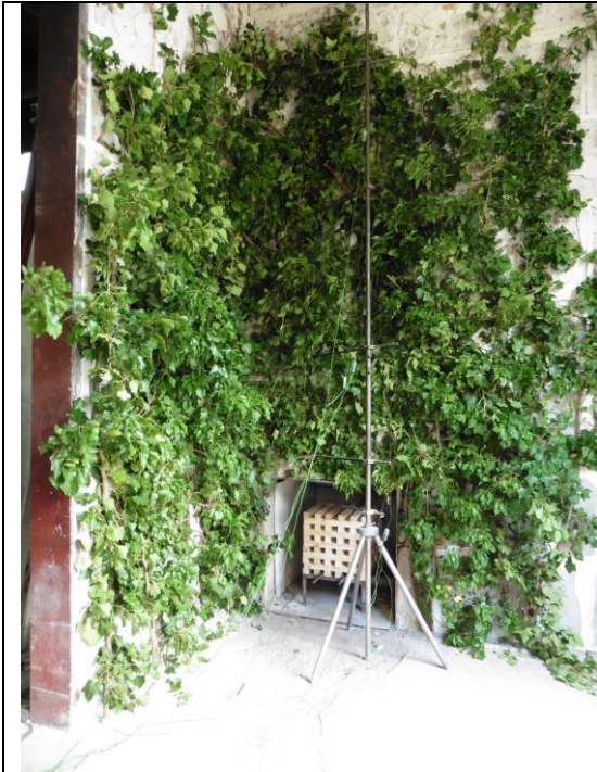
Figure 2-1: Ivy on the test bench of the MA 39 before the facade fire test
