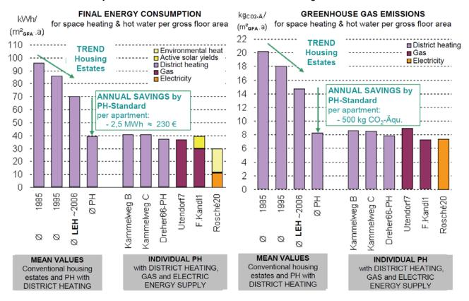
Space heating and hot water - final delivered energy and greenhouse gas emissions. Greenhouse gas factors: district heating 192 kg/MWh, fossil gas 250 kg/MWh, electrical energy 617 kg/MWh
