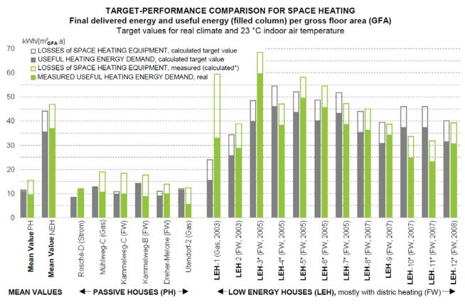
Target-Actual-Comparison for space heating. Final delivered energy and useful energy
